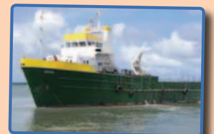
M.V. ORION UNDER REPAIR AT CLAXTON BAY L 51.66M X W 11.89M X D 5.5M ENGINES - 4 UNITS AT 1,050 H.P.
