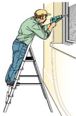
Figure 2b Correct - steps facing work activity
